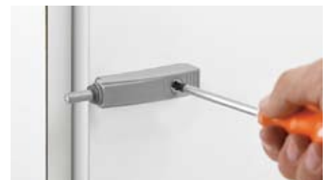
The ideal location for the TIP-ON unit (as shown above) is no more than 12" up the side panel or no more than 1/4 of the door width from the edge.
